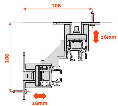
Front adjustment of one upright profile involves lateral displacement of the other.
