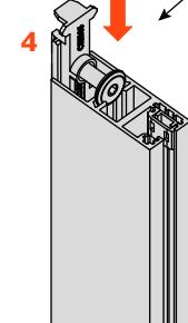
Lock the fixing element in the profile, observing the dimensions indicated by the configurator
