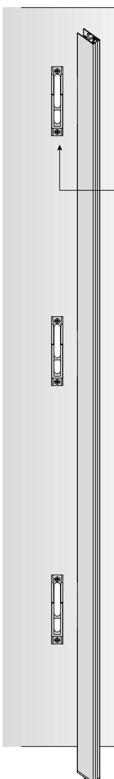
Loosen the screw and remove the wall fixing element
